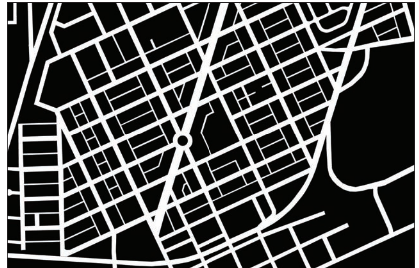
Example of connected street grid system in Old Town Ranson. Intersections per square mile: over 300.
